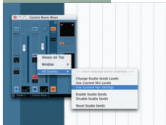
The Control Room mixer enables you to set up separate, assignable sends.
