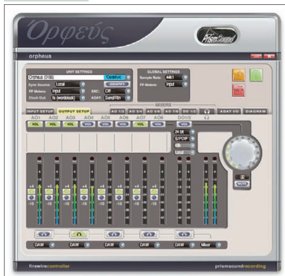
The control panel software provides control over the primary functions and settings. Each output can have its own low-latency mix configured.
