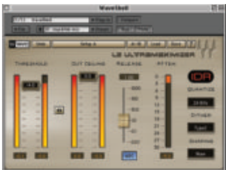
L2 Ultramaximizer. The Waves Ultramaximizer is a real crowd pleaser, increasing the loudness of a mix with no obvious unwanted artefacts. Unlike the L1, the L2 features an Automatic Release Control (ARC).
