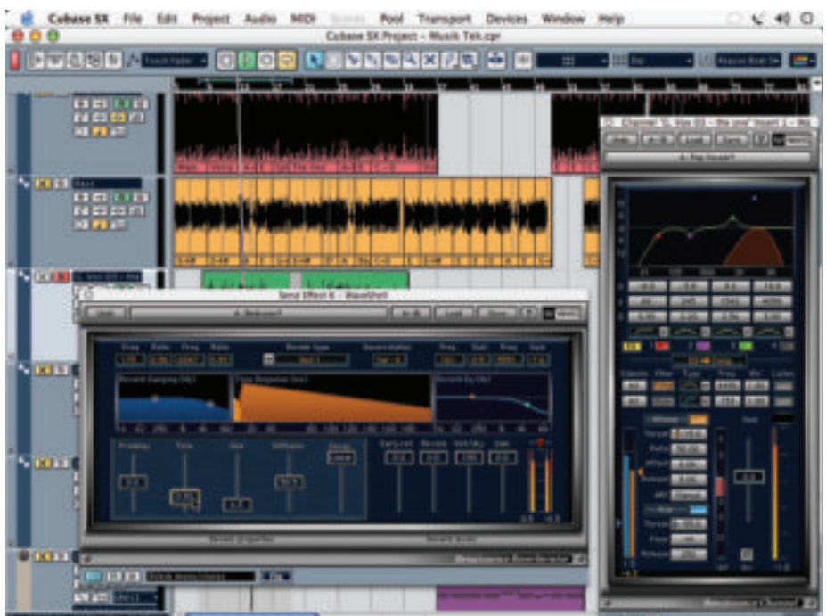
Ren Rev + Channel: Cubase SX utilises the OS X-compatible VST plug-ins Renaissance Reverberator (middle) and Renaissance Channel (right). Each has interactive graphic displays.
