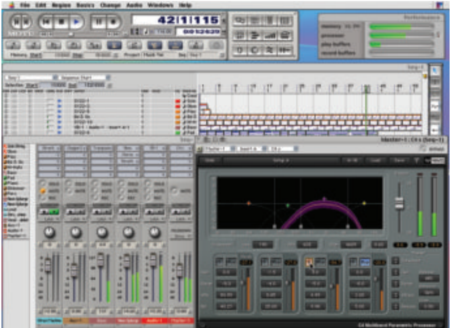
C4 solo DP: Digital Performer's own MasterWorks is a useful multi-band compressor, but the C4's graphics go one better. Here the display reveals the frequency spectrum affected by a solo'd compressor band.
