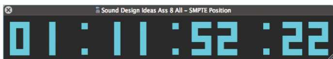
SMPTE timecode is represented in Hours : Minutes : Seconds : Frames. Timecode formats were defined by the Society of Motion Picture Television Engineers (SMPTE).
